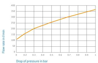
The flow diagram refers to the blocking variant with a maximum gap between socket and pin piece of  $\leq 0.5$  mm. The pressure reduction increases in the event of a changed gap measurement.
