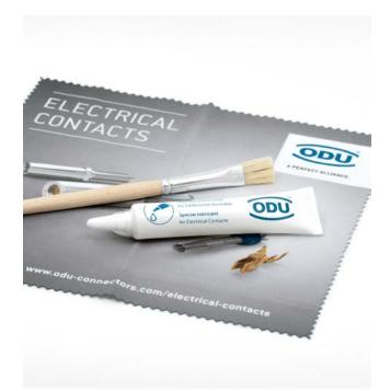
Contact lubrication improves the mechanical properties of contact systems. Cleaning the contact surfaces prior to lubrication is also recommended in order to remove pollution. With appropriate care, wear due to high mating frequency can be significantly minimised and the mating and unmating forces reduced. The cleaning and lubricating interval must be individually adapted to circumstances and should only be carried out with products recommended by the contact manufacturer.
