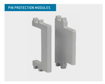
For connections with small pin diameters, these modules serve as protection for the pins. Especially in the case of small contact diameters ( $\emptyset$  0.76 / 1.02 mm), pin protection modules provide additional protection against unintentional bending of the pins.
