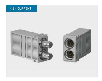
Contact diameter: 8 mm Mating cycles<sup>1</sup>: minimum 100,000 Current-carrying capacity<sup>2</sup>: 142 A
