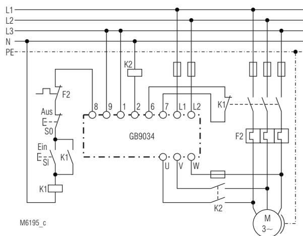
Fig. 1: Schematic diagram for a motor with electronic braking
