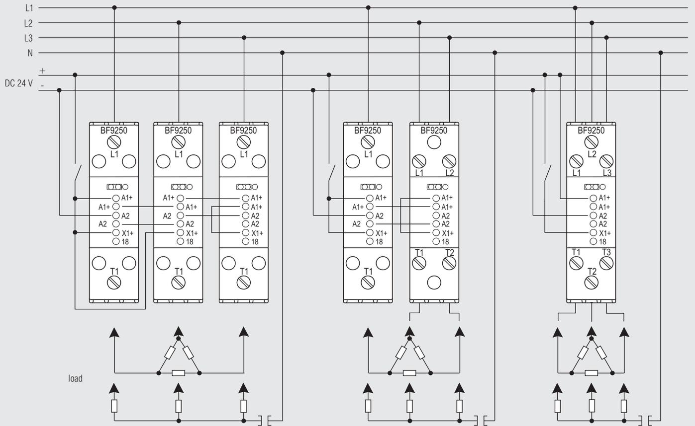
3-phase load switched by 3 single-pole semiconductor contactors
