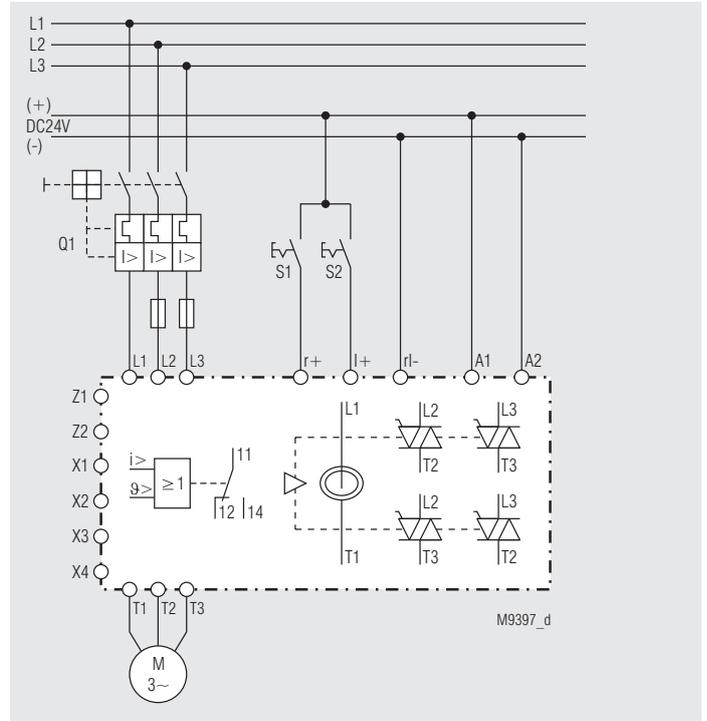
BH 9255 with A1/A2 = AC/DC 24 V and control input AC/DC 24 V or DC 24 V
