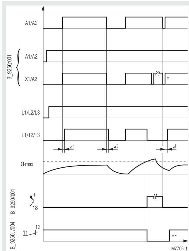
\* The latching function of the overtemperature monitoring is resetted by disconnecting A1/A2 for a short moment
