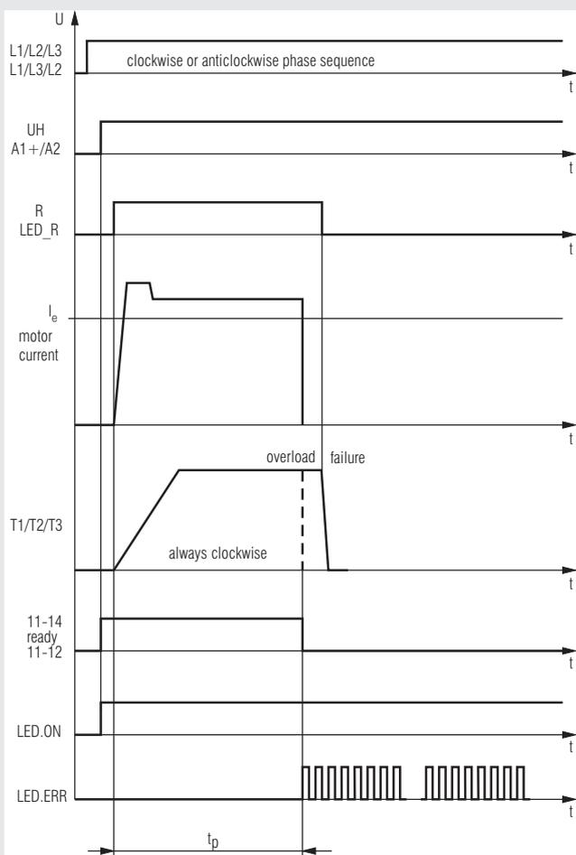
$t_p$  = overload response time according to characteristic class 10A or 5
