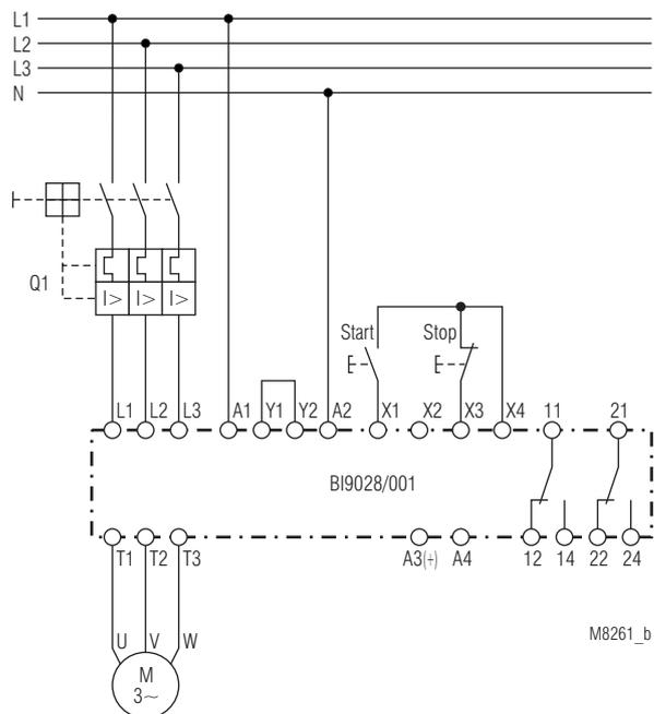
**Fig. 2:** Schematic diagram for softstart-brake combination
